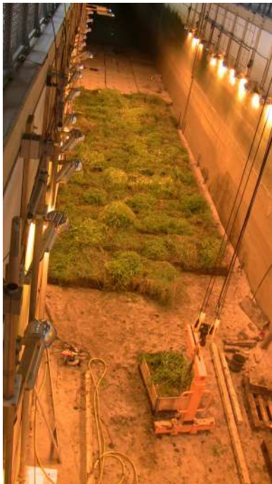
Building a saltmarsh in the Large Wave Flume (Grosser Wellenkanal, GWK) of Forschungszentrum Küste (FZK) in Hannover, Germany, to test over-marsh wave energy dissipation under storm waves. The flume is 330 m long, 7 m deep and 5 m wide. Photograph by Tom Spencer.
